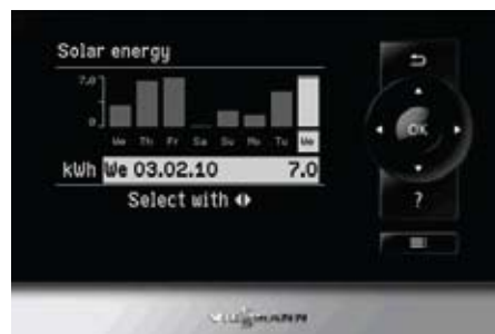
Vitotronic 200 HO1A Weather compensation control (Illustrates solar yield when linked to solar system).
